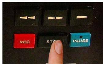
Stop (Tape motion ceases, mode is released.)
