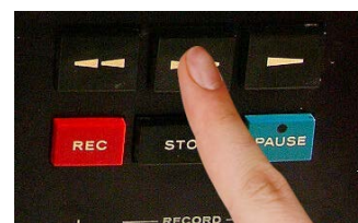
Fast Forward (Tape winds rapidly onto right reel)
