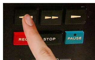
Fast Rewind (Tape winds rapidly onto left reel)
