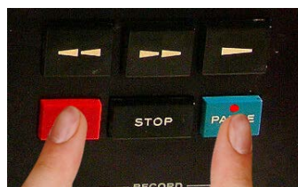
Record Pause (Establishes Record mode without starting tape movement, RECORD MODE switches must be ON, both lights illuminate.)
