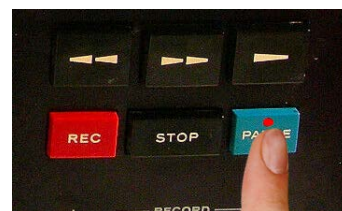
Pause (Stops tape motion; when recording retains mode and light illuminates; during Playback acts as a STOP button.)
