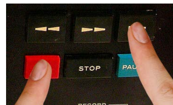
Record (Tape is recorded, MODE switch must be ON.)
